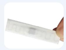
LinTRAK<sup>®</sup> Linen RAIN<sup>®</sup> RFID (UHF) Tags withstand the rigors of repeated washings, including exposure to water, cleaning chemicals, sterilizing heat, and water extraction pressure. The patented design securely positions the inner chip relative to the antenna, which guarantees consistent performance over the life of the tag.
